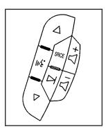
The audio steering wheel controls may be different depending on your vehicle's options. Some audio controls can be adjusted at the steering wheel. They include the following:
